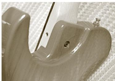
Yeah, the "Tone Socket." I always dug the way the ol' interlock worked and wanted to do it in a way that would be a bit easier to use and a bit more of a traditional wood to wood joint. It consists of brass pieces that are placed flush in the neck and body,
